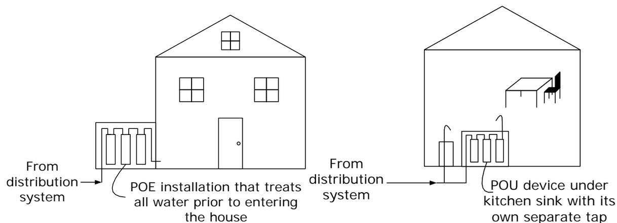
**Figure 1. Typical Installment of POU and POE Systems**
