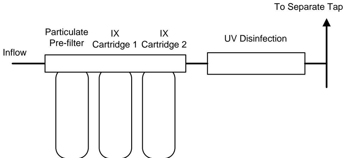
**Figure 4 Sample Topology of a Potential POU Ion Exchange Treatment Train**
