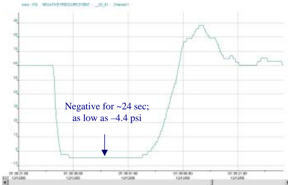
Figure 7. Distribution System Pressure Monitoring Following a Pump Station Power Outage. A) Daily monitoring data, B) Enlargement of the negative pressure event.
